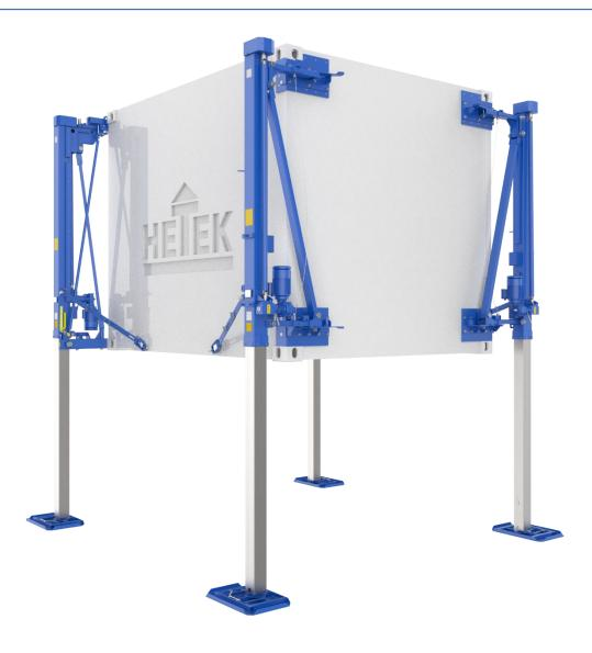
Container lifting system type for 273 radar shelter. Special mechanical solutions enable high rotational and translational stiffness which is necessary for the proper operation of the 3D radar. Terrain inclination up to 7° are possible with a lift height of 1.85 m. The lifting system is equipped with automatic position control and a CAN bus interface for integration into the Shelter control console.
