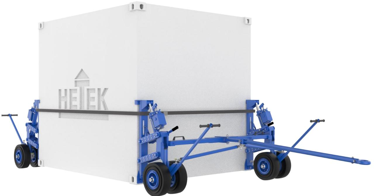
Lifting wheels series 507 up to 500mm stroke are suitable to move containers or modules up to 17t on little paved and lesser levelled ground. The assembling is to the frontside into the ISO corners, when the container is on standing the ground. To traverse the container has to be lifted up hydraulically by means of lifting wheels and can be moved from different vehicles. Using lifting wheels also small containers and structures can be loaded into cargo planes.
